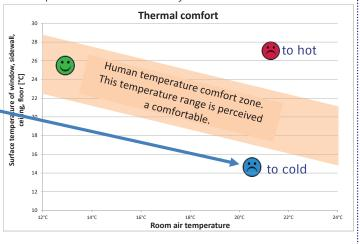
With the Cello<sup>®</sup> Heating Panel you can influence the temperature of both the air and the surfaces in a given space. The optimization of both parameters at the same time allows you to provide a comfortable ambiance even at a low room air temperature.
